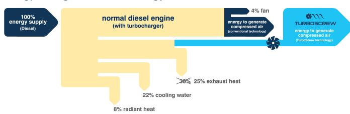
Using the TurboScrew technology, the engine delivers approximately 14% more energy to the compressor than conventional technologies (measured under full load condition).
