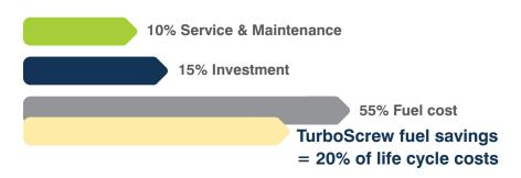
Based on average site running conditions, over lifetime of 10,000 hours, fuel savings of up to 30% can be achieved when compared with equivalent conventional compressors of this output range. This represents up to 20% of total life cycle costs.
