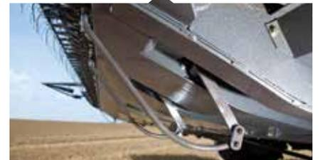
AutoLevel table control is available as an option with cutting height control. Smooth transition from one side to the other maintains a constant cutting height with sensitivity, as a result of quality hydraulics and electronics working together.
