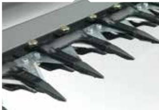
The Schumacher knife is the best performing knife in the business at 1,254 cuts a minute. Self-cleaning and consistently sharp, this keeps the crop moving in tough conditions.
