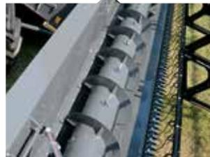
Full width auger fingers on the FreeFlow table increase auger throughput, ensuring positive and fast feed into the main crop elevator.
