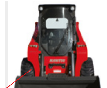
● Between-the-tire Design keeps machine length short and compact. Model 1900 R
