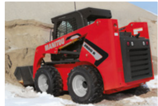
● Over-the-tire Design provides wider access and improved visibility. Models 2200 R and 2600 R
