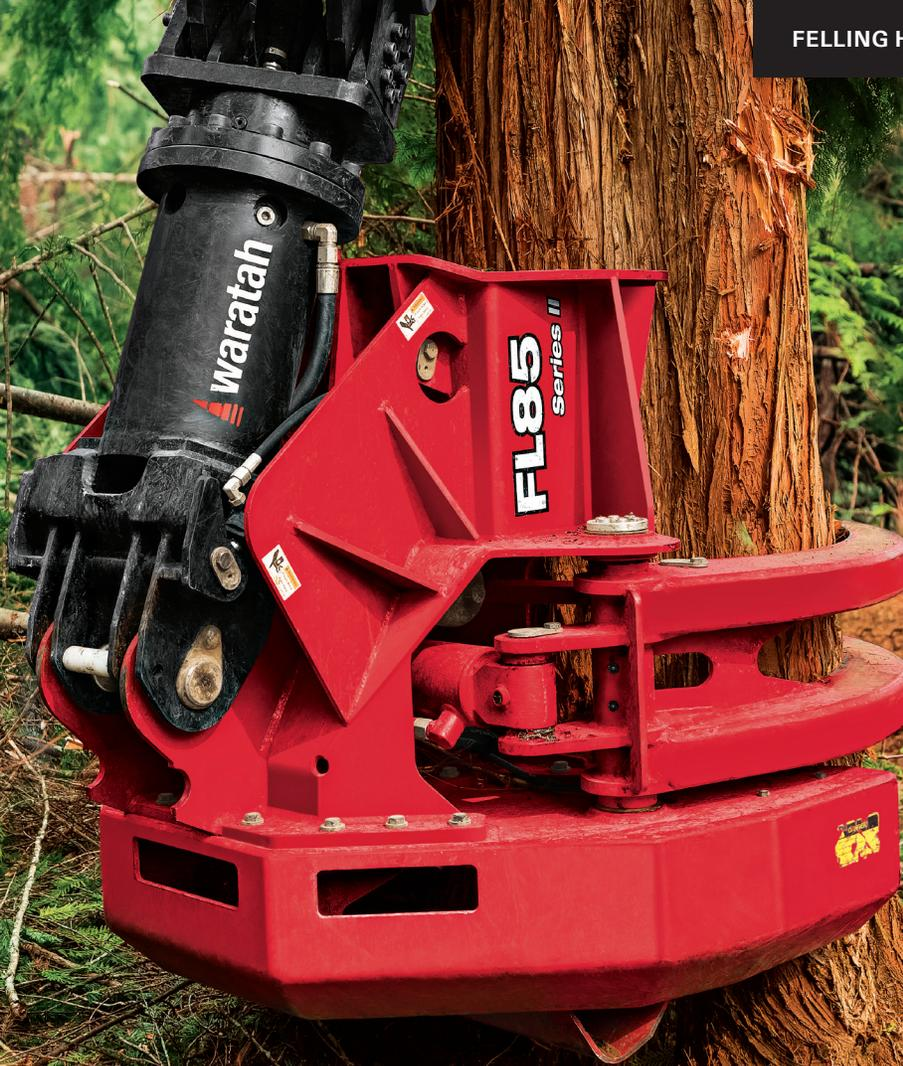
The versatile FL85 Series-II is a triple threat, working as a felling head, grapple and saw – all in one. Its large grapple and cutting capacities provide additional productivity-boosting advantages, and it's ideal for steep slope applications.
