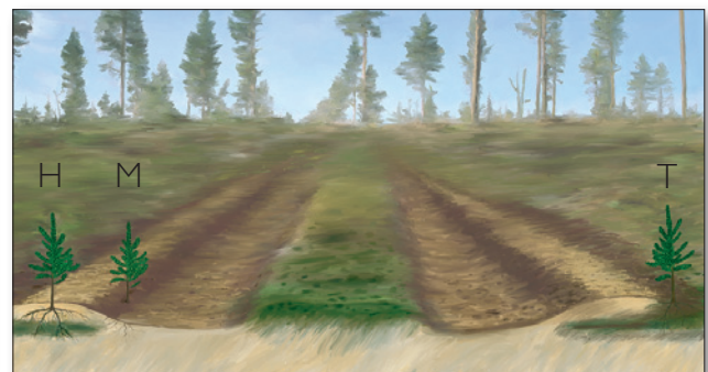
Bracke T35 creates planting spots with inverted humus layer (T), Mineral soil mounds on inverted humus layer (H) Mineral soil mounds on mineral soil (M).
