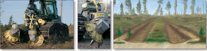
The Bracke T26.a creates planting spots with inverted humus (T), mineral soil mounds on inverted humus (H), and mineral soil mounds (M).
