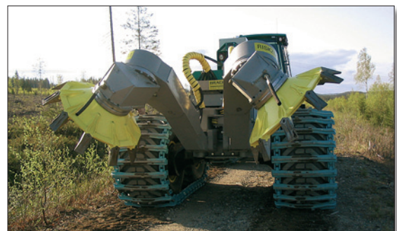
The Bracke S35.a can be attached to a one-, two-, or three-row moulder.
