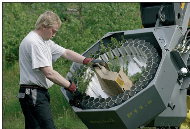
The planting tube and carousel are available in several different sizes.
