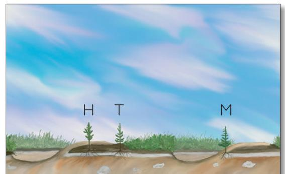
The Bracke M46.a creates planting spots with inverted humus (T), mineral soil mounds on inverted humus (H), and mineral soil mounds (M).
