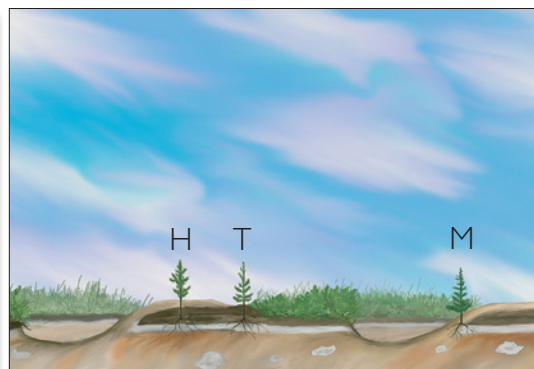
The Bracke M36.a creates planting spots with inverted humus (T), mineral soil mounds on inverted humus (H), and mineral soil mounds (M).
