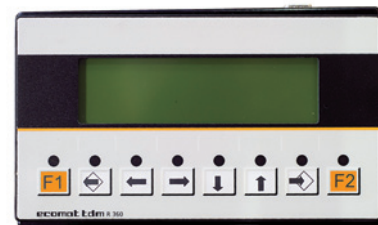
At the heart of the M36.a lies Bracke Growth Control, a PLC-based control system using CAN-bus technology.
