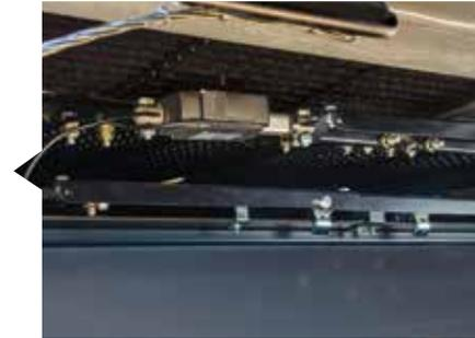
Electric Sieves operated from the cab enable easy attention to the sample, high sieve dividers give increased output on undulating land.
