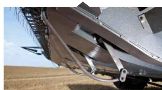
AutoLevel table control is standard with cutting height control. Smooth transition from one side to the other maintains a constant cutting height. Coupled with the Automatic reel speed feature, making table control easy on the operator.
