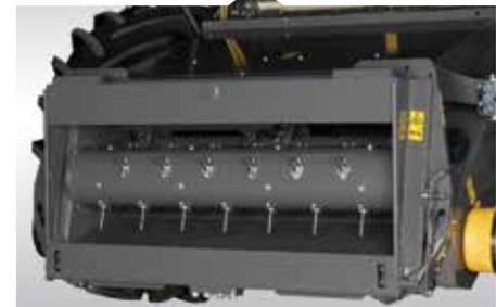
The Power Feed Roller at the front of the main crop elevator gives a consistent crop flow from the table into the main crop elevator. It can be reversed simply and effectively from the cab.
