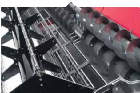
The optional rape auger for the PowerFlow table increases the flow of tall crops into the elevator thereby increasing the output considerably. Two electrical side knives are available as options complete the Rape seed kit.
