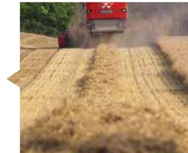
For those that require straw, the threshing system is gentle and leaves the straw in perfect condition for baling feed and bedding straw or producing products for power generation.
