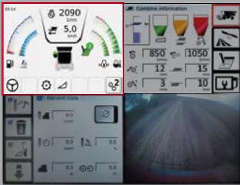
The **General information screen** is always on display in the top left hand side corner of the terminal. It shows engine speed and ground speed. Alongside these are the gauges for fuel, AdBlue, oil and engine temperature. The graphic also displays the current combine status for the grain tank and the unloader.
