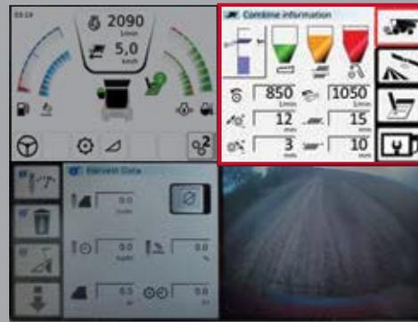
The easy to read displays on the **Combine main menu** indicate actual and set header height, grain loss from straw walkers and sieves and the returns volume. Below that current settings for header height, cylinder speed, concave opening front/rear, fan speed, sieve opening top/bottom. Through short cuts keys on the icons all settings can quickly be adjusted.
