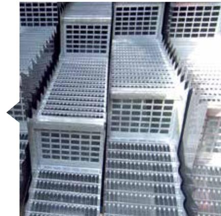
The long straw walkers feature four steps with 'active walls'. The 210 mm high, vertical sections of the walker steps are made up of permeable grids. These are the highest for any conventional combine. The front steps of the straw walkers are reinforced for maize harvestmaking the combine much more durable for variable crops
