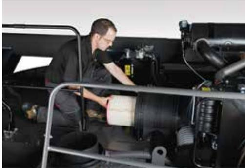
Checking and cleaning the air filter
