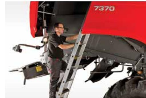
Safe engine compartment and grain tank access with removable ladder
