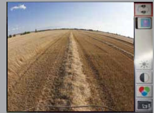
Up to two **Camera views** can be seen in the terminal windows at the bottom. The operator can decide to have the camera view on display at all times or only for example, whilst reversing. The image can be enlarged to show the whole screen at the touch of a button, quickly and safely.
