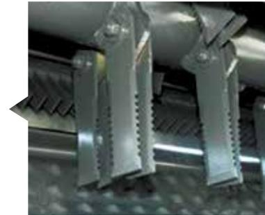
An adjustable dimple plate is standard to make sure straw is chopped consistently.
