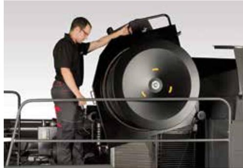
Safe and simple access for radiator cleaning
