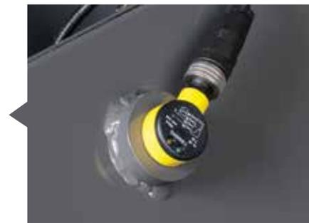
A simple returns sensor displays volume in the cab and enabling quick changes to improve the sample.
