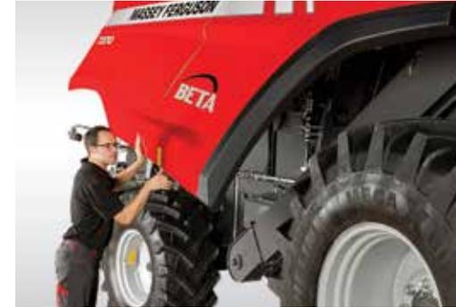
One piece panels with lights allow for quick inspection access
