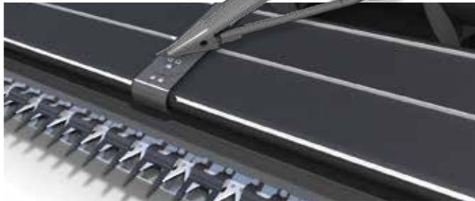
The knife is a massive 1.14m from the table auger so vision and performance are optimum. The rugged PowerFlow belts power the crop away from the knife and into the main crop elevator at a consistent speed. The belts also deflect stones rather than taking them into the machine where they might cause damage.
