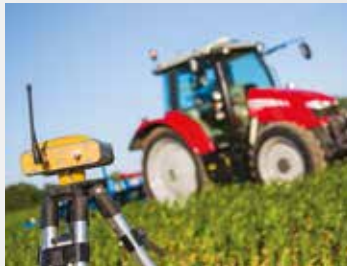
RTK Base Station
