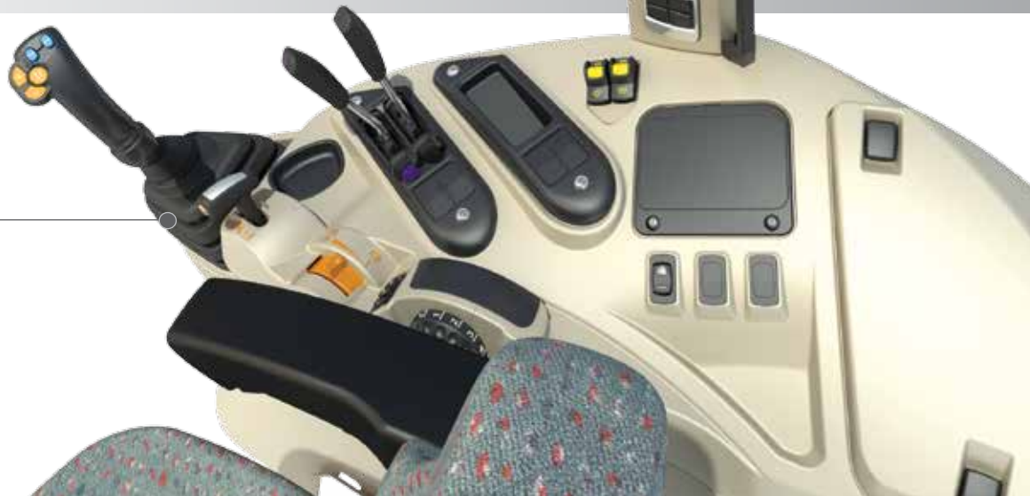
Mechanically controlled Multi-function loader joystick
