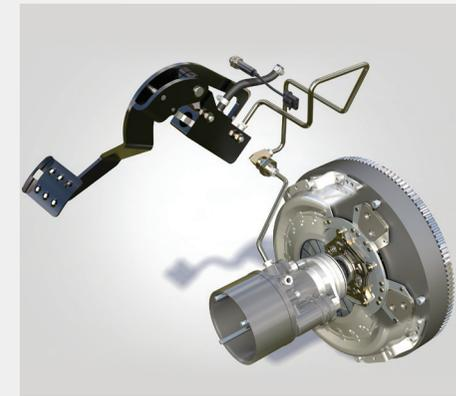
As the transmission is new, Massey Ferguson's engineers have been able to design the clutch pedal lever operation with the customer comfort in mind. This new design allows a lower effort so that shifting becomes as smooth as in any modern car.
