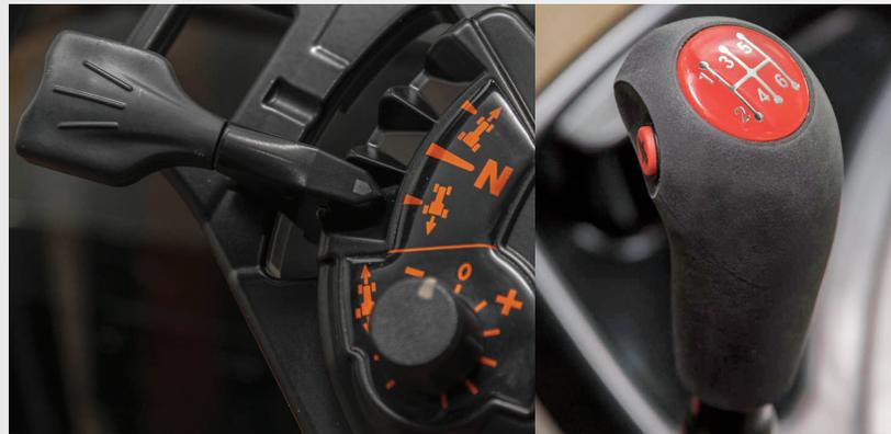
The optional left hand Power-Control lever provides convenient three-in-one, straightforward operation through the state of the art transmission. The operator can shuttle between forward and reverse and select neutral. For greater accuracy, shuttle responsiveness can be adjusted using the Comfort Control selector, the ultimate combination for working with a front loader.
