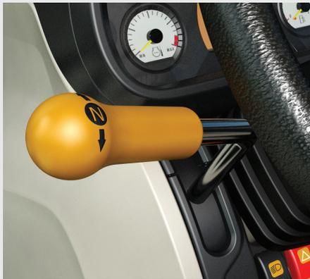
Moving between forward and reverse at field headlands or around the yard, or when hooking up implements, is made easy with a mechanical synchronised shuttle lever mounted on the dashboard.
