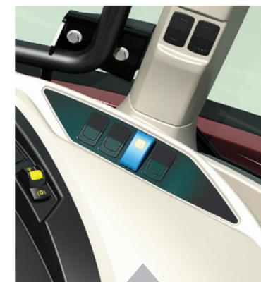
New 100 litres/min 'Combined' flow option at the press of a button
